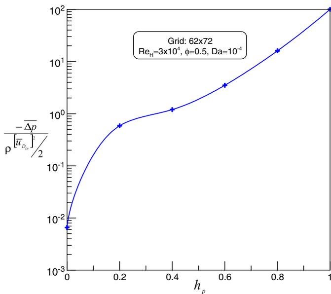
Fig. 4. Pressure drop as a function of porous layer thickness  $h_p$ .
