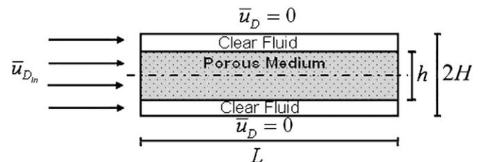
Fig. 1. Channel with porous layer.
