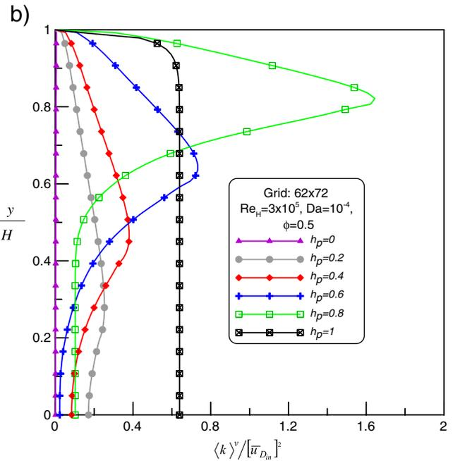
Fig. 3. Effect of porous layer thickness  $h_p = h/H$  (see Fig. 1): a) non-dimensional mean velocity, b) non-dimensional turbulent kinetic energy.
