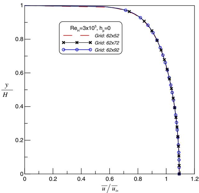
Fig. 2. Effect of grid size on velocity field.
