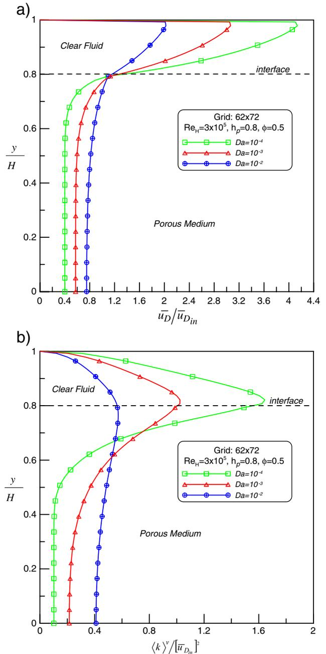
Fig. 5. Effect of  $Da$  on: a) mean velocity, b) turbulent kinetic energy.
